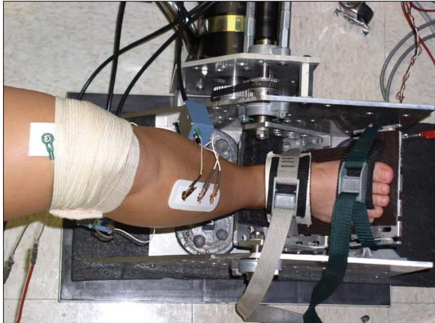
**Figure 2.** The seated subject's leg is positioned in the stepper motor testing apparatus with the foot strapped to the foot plate and with a knee angle of 130 degrees and an ankle angle of 90 degrees. Electromyogram electrodes are visible on the subject's tibialis anterior. The electric motor (top) imposes a rapid dorsiflexion (5 degrees in 50 ms), which elicits the stretch reflex. The H-reflex is elicited by electrical stimulations of the tibial nerve.
